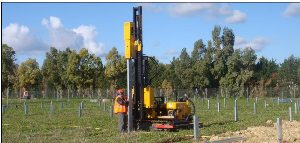
Figure 5: Sonnette de battage hydraulique
