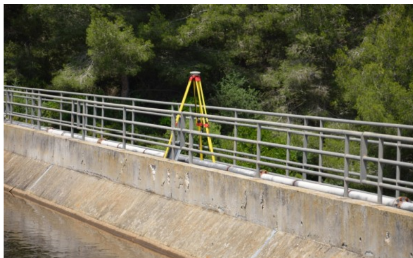
Figure 5 : Base GPS RTK fixe Leica 1200
