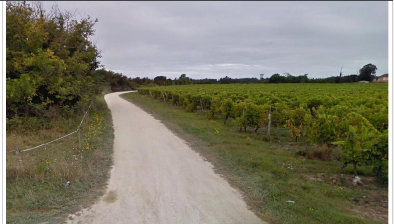
FIGURE 19 : EXEMPLE DE VOIE EN SITE PARTAGEE EN BICOUCHE CALCAIRE AVEC DES MODES DE DEPLACEMENT DOUX
