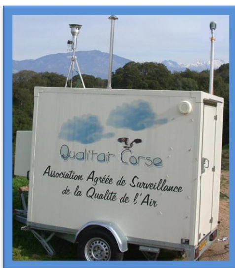
Figure 4 : Station mobile : la remorque
